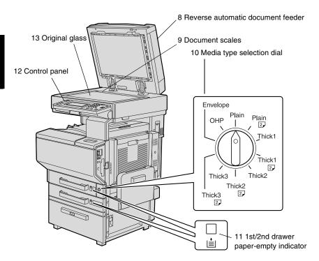
\* The illustration above shows the reverse automatic document feeder and large-capacity paper feed cabinet installed.
